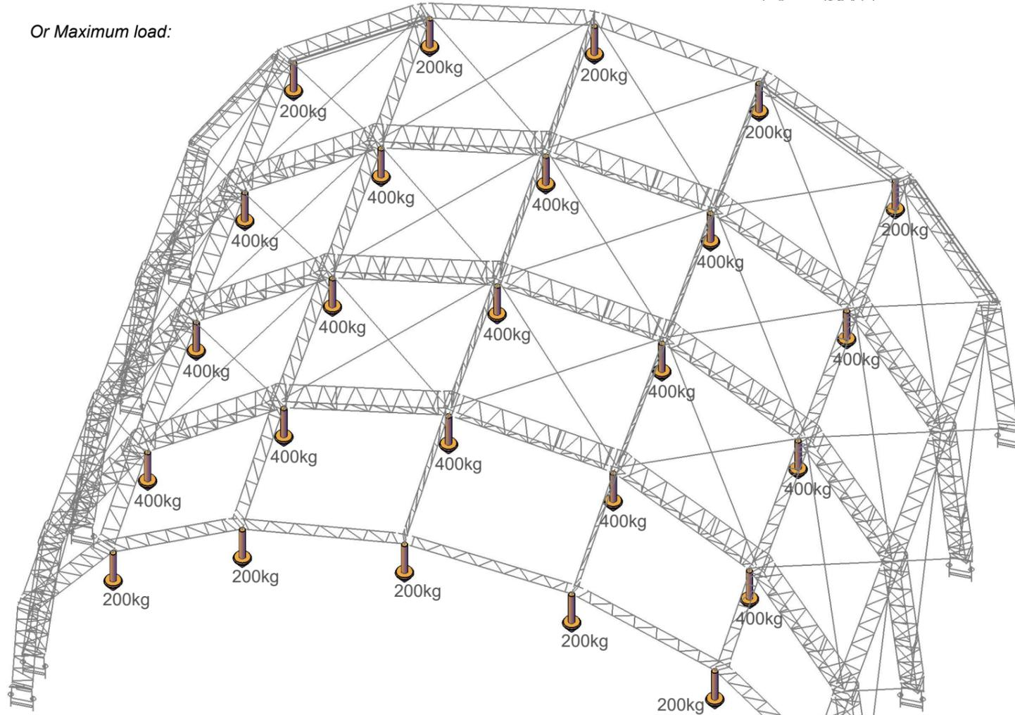
Based on: ALC Truss Tunnelstage 20x 17m
